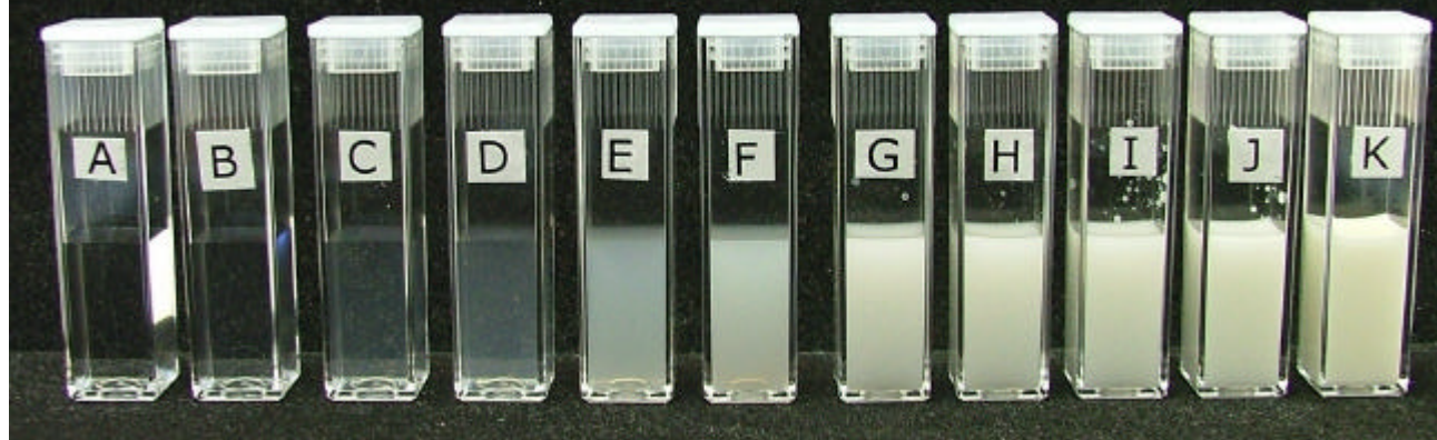
Figure 4: Photograph showing the various concentrations of Intralipid that were used in figure 2. The concentrations of the Intralipid samples were A = 0.0001% w/v, B = 0.001% w/v, C = 0.005% w/v, D = 0.01% w/v, E = 0.05% w/v, F = 0.1% w/v, G = 0.5% w/v, H = 0.75% w/v, I = 1% w/v, J = 2% w/v and K = 10% w/v (neat sample). The zeta potentials of samples A to I were successfully measured in the Nano i.e. up to 1% w/v concentration.
